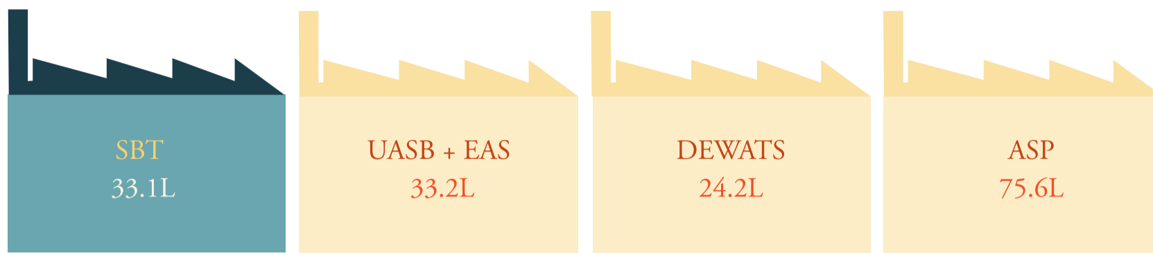
Total Cost of Ownership (TCO) for 15KLD plant, with a lifetime of 25 years and land cost of Rs 2,200/m 2 (Rs lakh)
